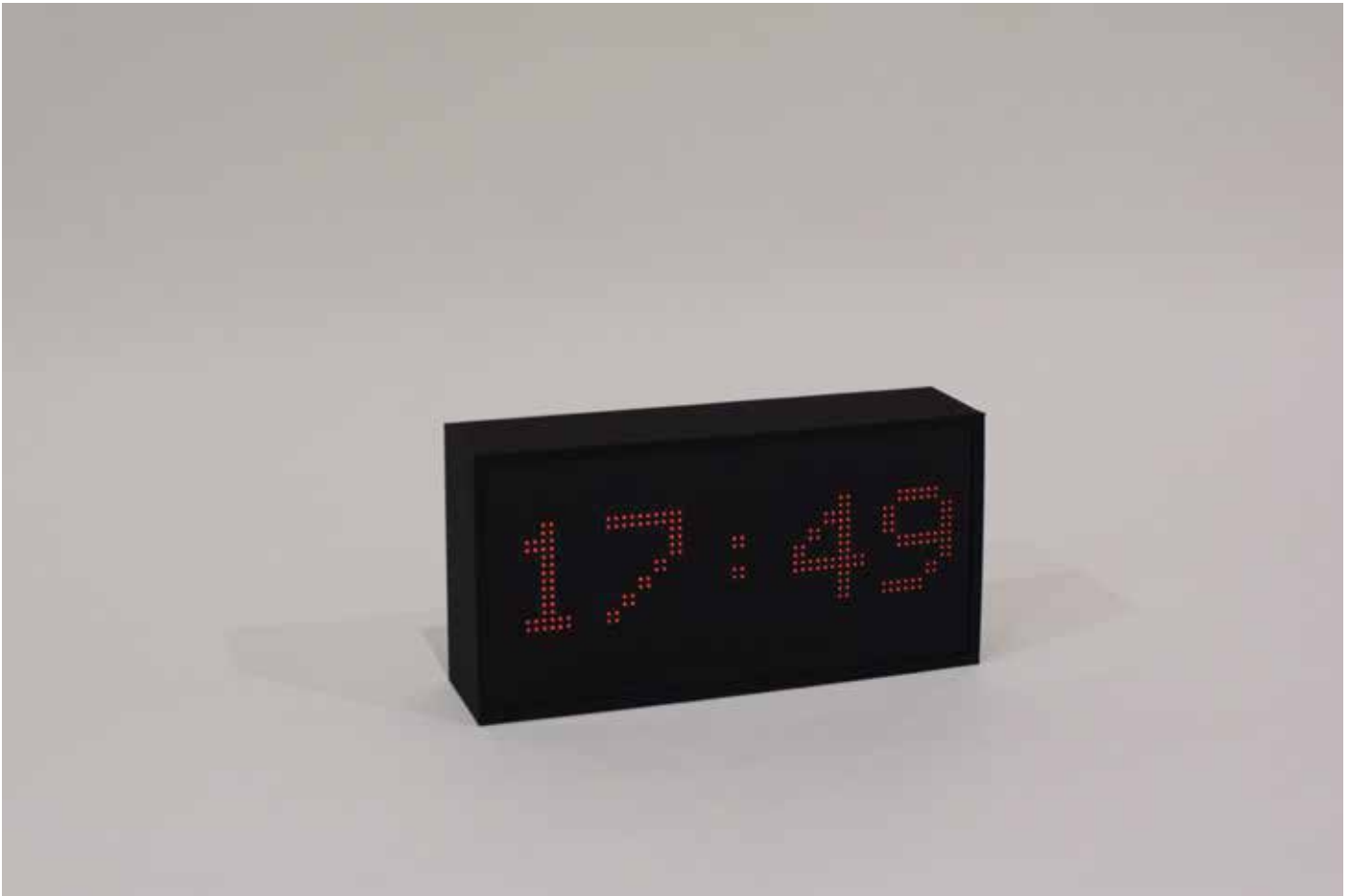
15.11.2025, 2026, LED matrix panel in a 3D-printed housing, controlled by ESP32, 20x10x5 cm
